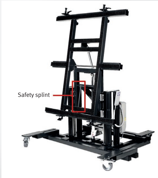
Figure 9: position of safety splint
